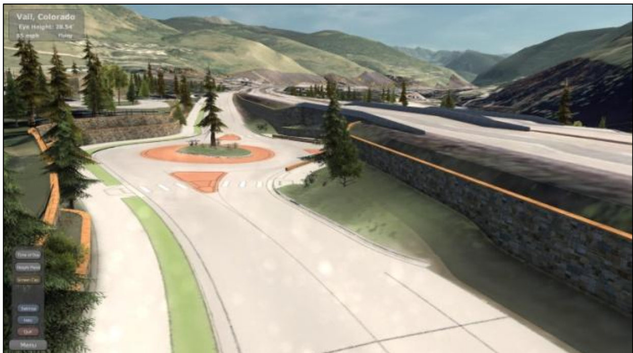
Proposed Simba Run Underpass without sound walls shown as viewed from North Frontage Road looking east.
